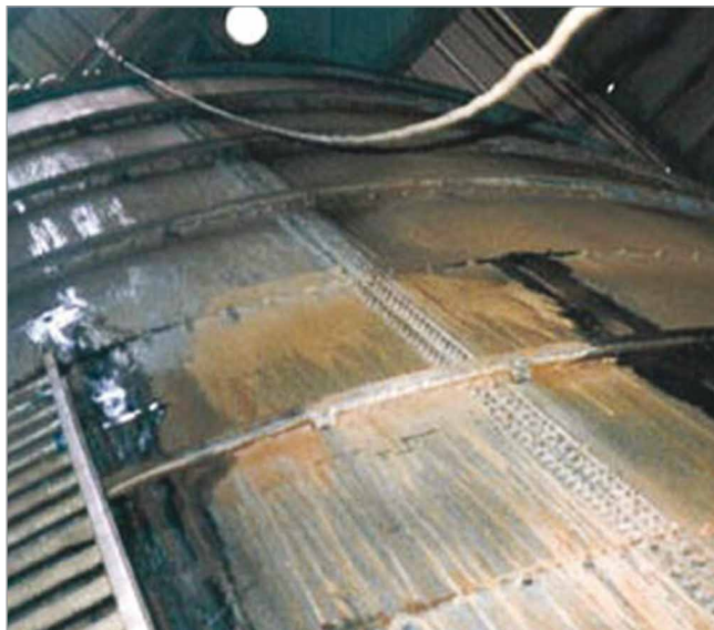
Holes created by chemical corrosion
